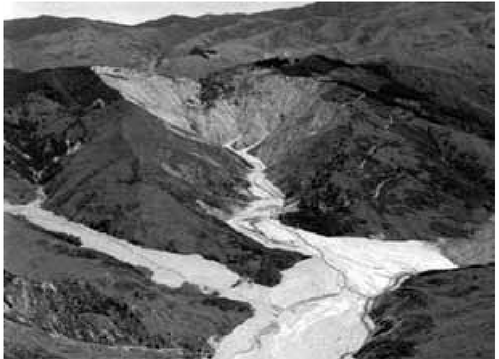
Figure 2: Tarndale Slip - erosion in the headwaters of the Waipaoa River where faulting has led to potentially unstable crush zones in the argillite rocks.
